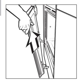
■ Lift up the door until the hinges disengage. Remove the door.
